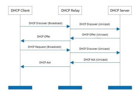
The working principles of DHCP Relay are as shown below.
