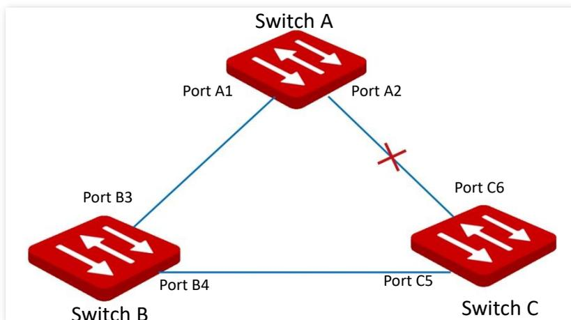
After calculation, switch A is selected as the root bridge, and the link between ports A2 and C6 is blocked.
