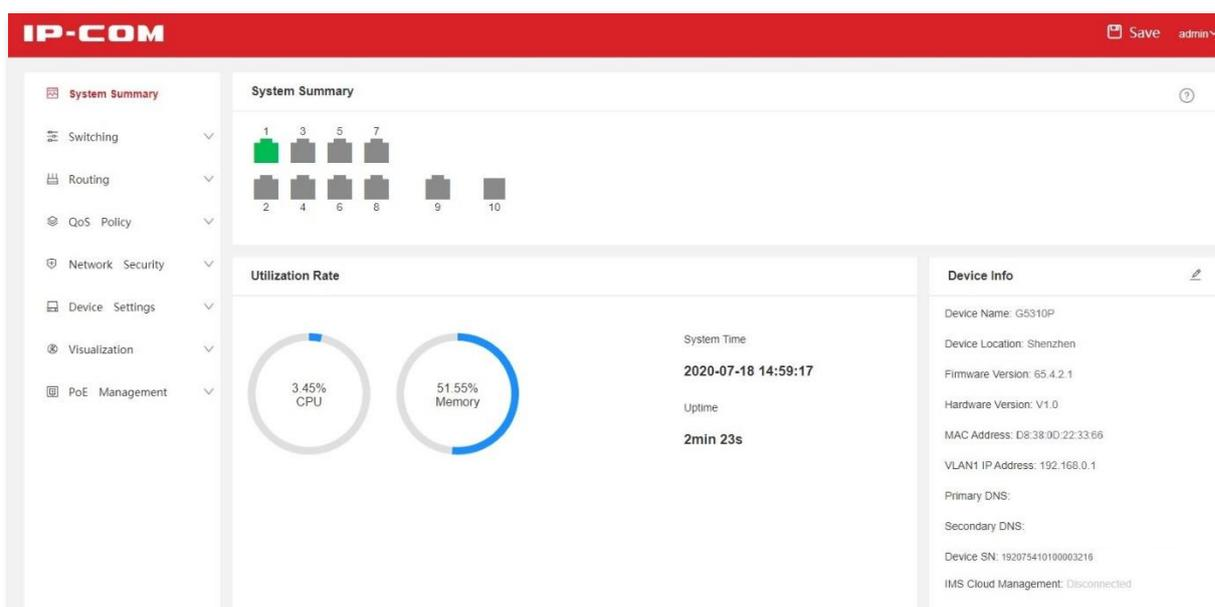
The image shows the IP-COM web UI dashboard. The top navigation bar is red with the IP-COM logo on the left and "Save admin" on the right. A sidebar on the left contains a menu with items: System Summary, Switching, Routing, QoS Policy, Network Security, Device Settings, Visualization, and PoE Management. The main content area is divided into several sections:
