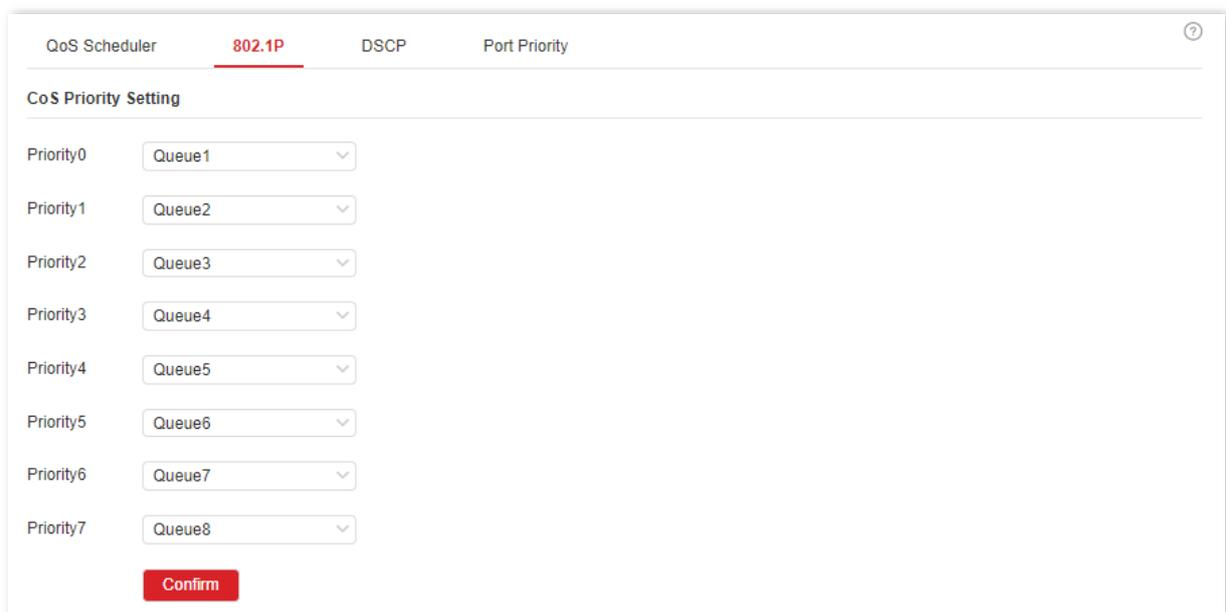
The screenshot shows the 'QoS Scheduler' configuration page for '802.1P'. The page has tabs for 'QoS Scheduler', '802.1P', 'DSCP', and 'Port Priority'. Under the '802.1P' tab, there is a 'CoS Priority Setting' section. This section contains eight rows, each with a priority label (Priority0 through Priority7) and a dropdown menu for selecting a queue (Queue1 through Queue8). A red 'Confirm' button is located at the bottom of the configuration area.
