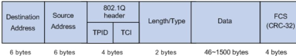
The figure below displays a detailed view of an 802.1Q tag. The field **Priority** under TCI is the 802.1P priority, which consists of 3 bits ranging from 0 to 7.
