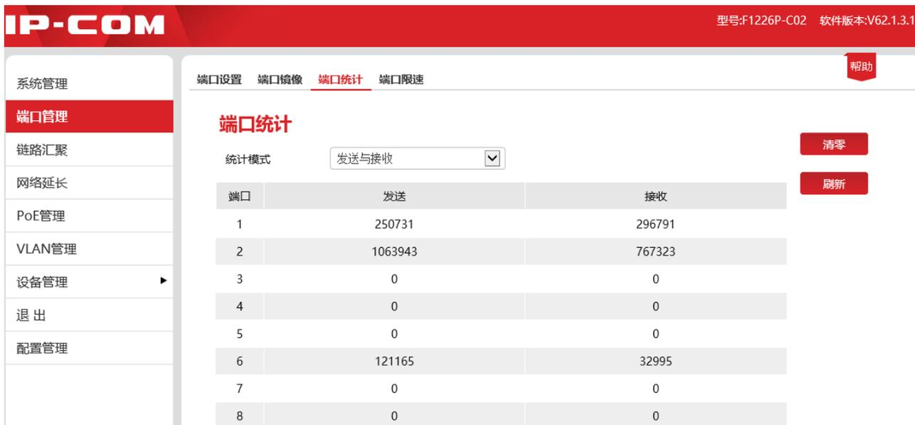
The screenshot shows the IP-COM web interface for port statistics. The page title is "端口统计" (Port Statistics). The navigation menu includes "端口设置", "端口镜像", "端口统计", and "端口限速". The "统计模式" (Statistics Mode) is set to "发送与接收" (Send and Receive). The table displays the following data:
